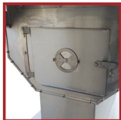
Side clean out door with air vent
